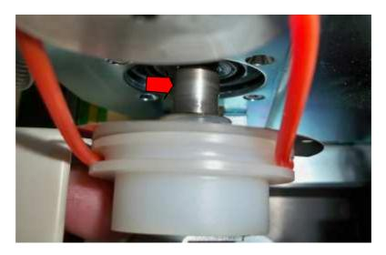
**6** Using an IPA (Isopropanol) soaked cleaning cloth, clean off any of the old grease on the shaft. There is just enough room to get the cleaning cloth in from the rear as shown below. With the cloth pressed against the shaft, turn the Black roller with your other hand;
