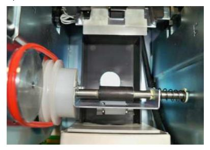
Position yourself on the right-hand side of the printer. Pull the metal flipper tray all they way towards you (compressing the spring all the way. Be careful to ensure the metal vane clears the front fascia. This may mean you need to rotate the flipper further than 90° (seen inset photo);
