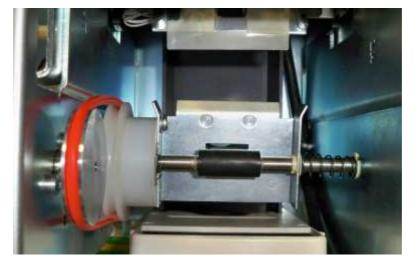
**3** Turn the flipper tray away from you so that it is at 90° (vertical). The Black rubber roller should be towards the rear of the printer.
