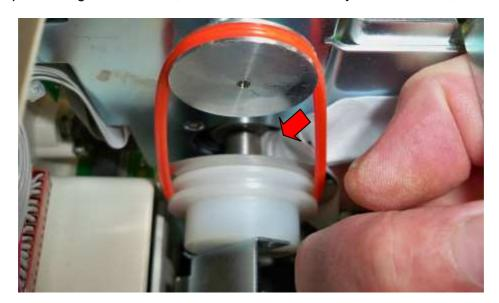
**7** Finally, using a small paint brush or similar, apply a <u>very small amount</u> of fresh general purpose grease onto the shaft;
